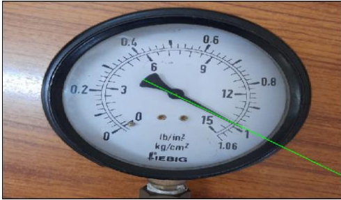
Fig. 4.3 Hough Line for the detection of the Pointer
