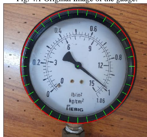
Fig. 4.2 Detection using Hough Circle Transform and 10-degree separations marking.
