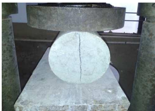
Fig 4: Tensile strength test for PFRC Cylinder
