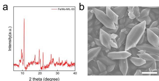
Figure 1 Material characterization of FeMo-MOF: (a) XRD; (b) SEM.
