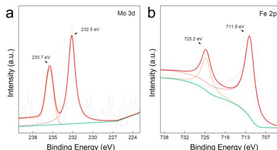
Figure 2 XPS characterization of FeMo-MOF: (a) Mo 3d; (b) Fe 2p.
