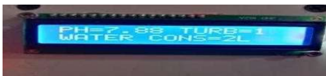
Fig. 3 LCD display output Water quality analysis and smart water meter using IoT.
