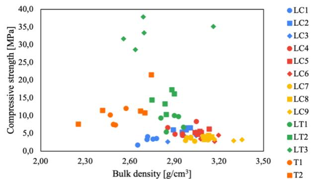
**Figure 8.** Compressive strength *versus* bulk density.
