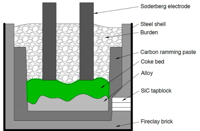
**Figure 1.** Schematic diagram of the submerged arc furnace [1].
