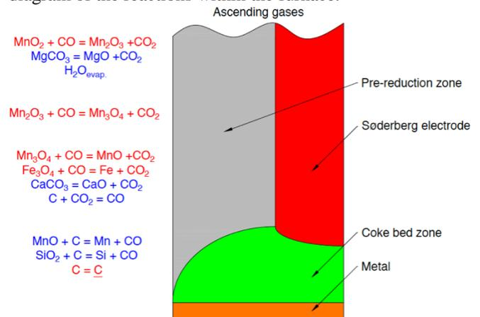
**Figure 2.** Main reactions in the submerged arc furnace [1]
