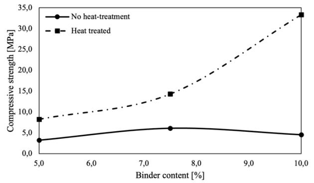
**Figure 6.** Compressive strength *versus* binder content and the influence of heat treatment.
