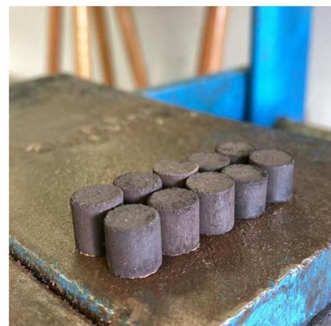
**Figure 4.** A batch of briquettes made with 0,250 mm top size raw material and 7,5 % of molasses.
