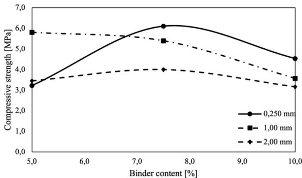
**Figure 5.** Compressive strength *versus* binder content.
