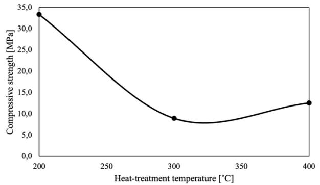
**Figure 7.** Compressive strength *versus* heat-treatment temperature.
