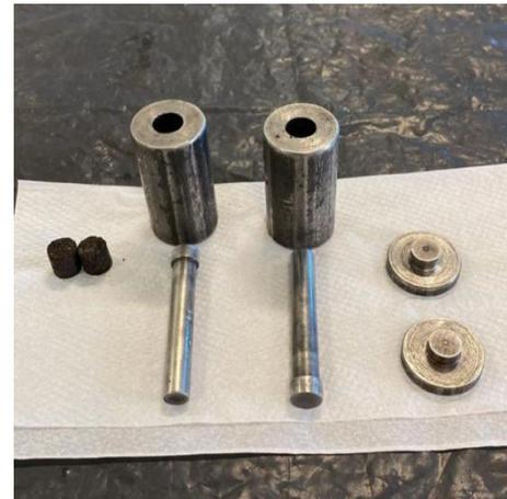
**Figure 3.** The cylindrical die and punch.
