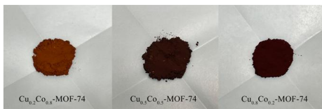
Figure 1 Morphology of the \text{Cu}_n\text{Co}_{1-n}\text{-MOF-74} materials.
