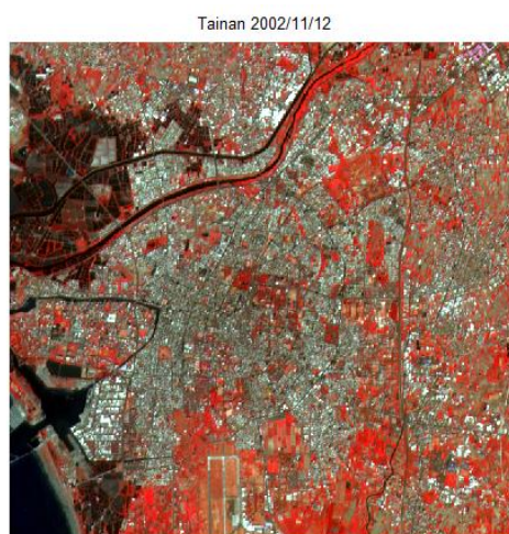
Fig. 1. SPOT satellite image over Tainan test site with false-color band combinations: near infrared (red), red (green) and green (blue).
