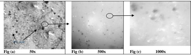
Fly ash is mixed with RTV silicone rubber shows good bonding between particles. Above microscopic analysis shows that there no bubbles found when Fly ash is mixed with RTV Silicone. Analysis is carried out at 50 X, 500X and 1000X respectively. Microscopic analysis show that RTV is mixed with fly ash which increase the mechanical properties.
