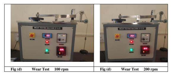
When a flexible pipe is laying on the seabed, it is exposed to a lot of corrosion and wear. Thus, we conducted wear tests to measure the weight loss and wear of silicon rubber mixed with fly ash under such environmental conditions. Below are the results.
