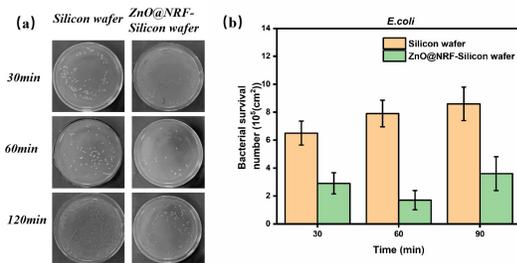
**Fig 4.** Photos of the bactericidal test on *E. coli*, the left figure (a) of the control silicon wafer is the picture of the coated plate, and the right figure (b) is the data statistical diagram
