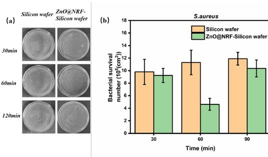
**Fig 5.** Photos of the bactericidal test on *S. aureus*, the left figure (a) of the control silicon wafer is the picture of the coated plate, and the right figure (b) is the data statistical diagram
