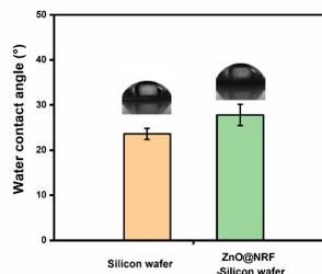
Fig 2. Water contact angle measurement of Control silicon wafer and ZnO@NRF on silicon wafer
