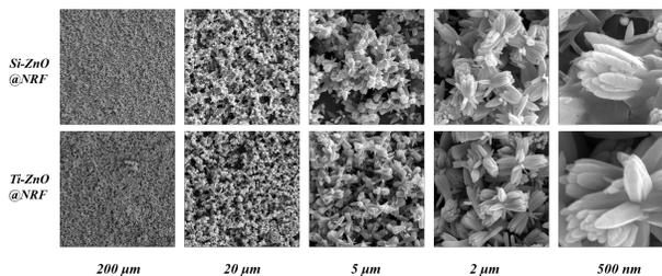
Fig 1. SEM images of ZnO@NRF of different sizes on silicon wafer and Ti wafer (The size range is 500nm-200µm)
