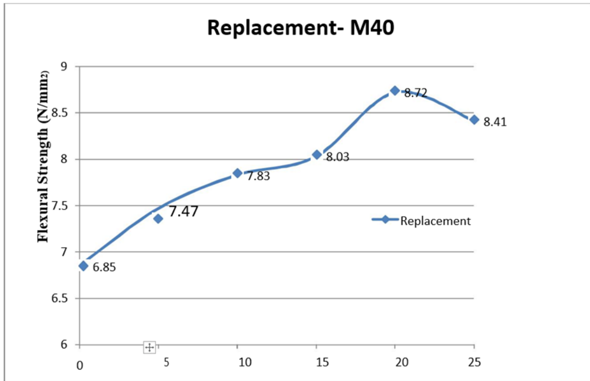
Fig. 2 Influence of ESP + CSA on Concrete of M40 Grade on Replacement for 28 Days Flexural Strength of Beam
