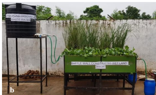
Fig 3. Baffle Wall Constructed Wet Land (BWCW) (a. Top view and C/S view, b. working model)
