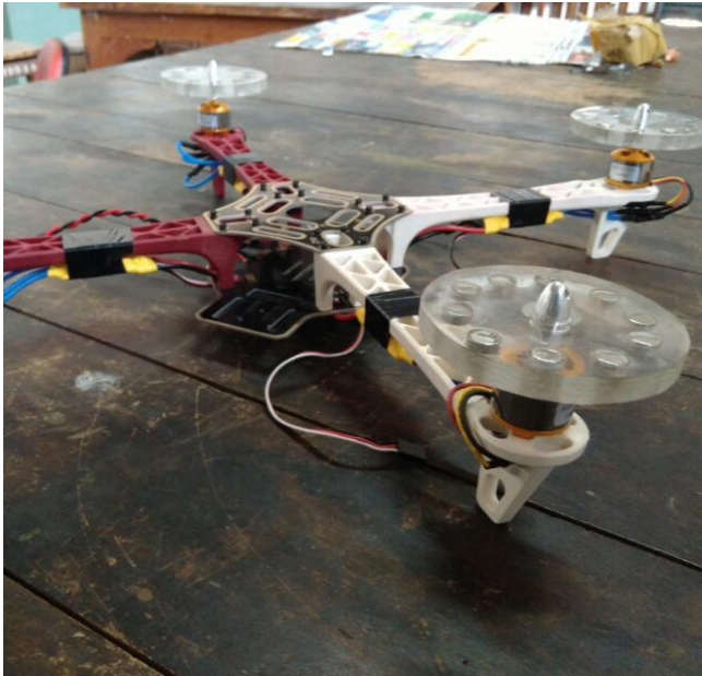
Fig. 10 : Prototype picture of the maglev system along with the 3D printed electrodynamic rotor
