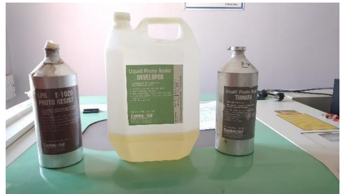
Fig.3. Photoresist and developing solution
