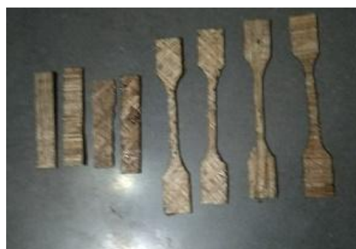
Fig.6 Tensile and Flexural Specimen.
