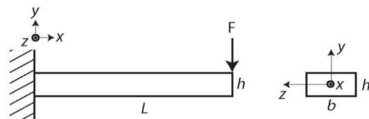
Figure 1: Cantilever beam under a concentrated load (F)
