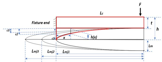
Figure 4: Parameters defining elliptical flexural hinge
