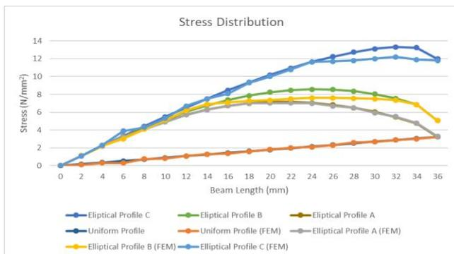
Figure 6: Theoretical and FEM beam stress
