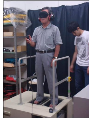
Figure. 4. Experimental scene for evaluation of the ankle joint sense on the motion-driven foot plate.
