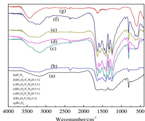
Fig.1 IR spectra of g-C<sub>3</sub>N<sub>4</sub>, Fe<sub>3</sub>O<sub>4</sub> and Fe<sub>3</sub>O<sub>4</sub>/g-C<sub>3</sub>N<sub>4</sub> composite catalysts.
