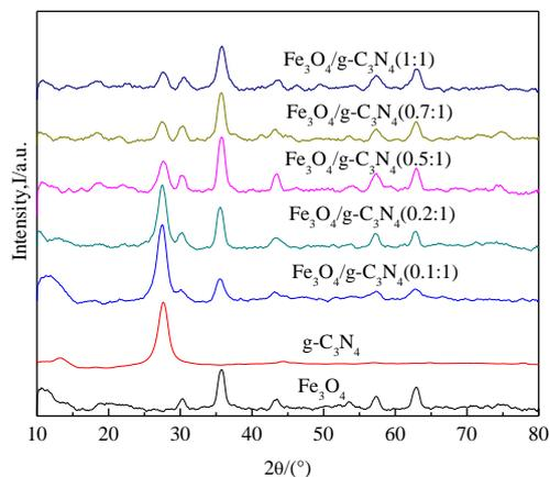
Fig.2 XRD patterns of g-C<sub>3</sub>N<sub>4</sub>, Fe<sub>3</sub>O<sub>4</sub> and different Fe<sub>3</sub>O<sub>4</sub>/g-C<sub>3</sub>N<sub>4</sub> composites.
