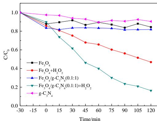
Fig.3 Photocatalytic performance of RhB by g-C<sub>3</sub>N<sub>4</sub>, Fe<sub>3</sub>O<sub>4</sub> and Fe<sub>3</sub>O<sub>4</sub>/g-C<sub>3</sub>N<sub>4</sub> composite in the presence H<sub>2</sub>O<sub>2</sub>.
