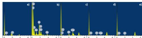
Figure 3. Energy Spectrometer (EDS) Elemental Analysis Image. a: clean titanium plate; b: hydroxyapatite coating; c-e: silver-loaded hydroxyapatite prepared at three AgNO<sub>3</sub> concentrations.
