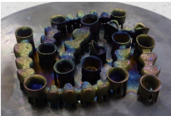
Fig. 2. View of base plate with prosthetic foundations after heat treatment in argon atmosphere
