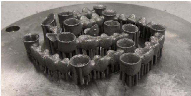
Fig. 1. View of the various prosthetic foundations with supports on the base plate directly after sintering process
