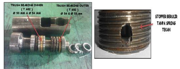
Fig. 7. Parts of the lateral coupling before improvement.
