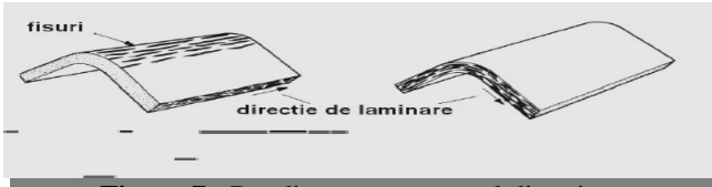
Figure 7: Bending on transversal direction
