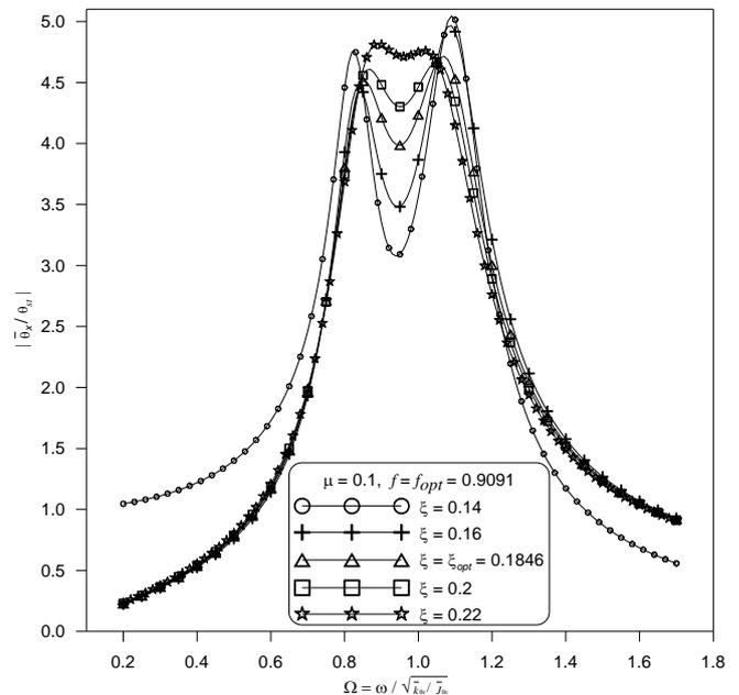
Figure 7 Influence of damping ratio ( $\xi$ ) of the two-dof vibration absorber on the dynamic magnification factor  $|\bar{\theta}_x/\theta_{st}|$  of the generalized main vibration system (see Figure 2(a)).
