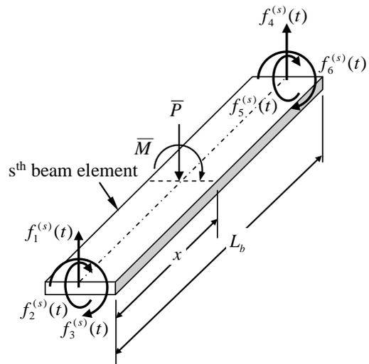
Figure 4 Equivalent nodal forces  $f_i^{(s)}$  ( $i=1$  to 6) of the  $s^{th}$  beam element due to a concentrated force  $\bar{P}$  and a concentrated moment  $\bar{M}$ .
