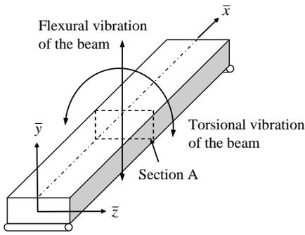
Figure 1 Flexural vibration and torsional vibration of a beam.
