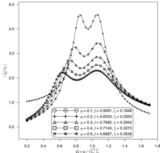
Figure 8 Influence of the ratio for mass moment of inertia ( $\mu$ ) of the two-dof vibration absorber on the dynamic magnification factor  $|\bar{\theta}_x/\theta_{st}|$  of the generalized main vibration system (see Figure 2(a)).
