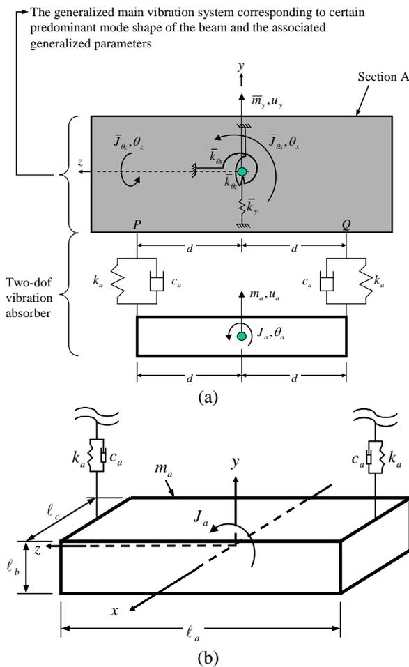
Figure 2 (a) The generalized main vibration system corresponding to certain predominant mode shape of the beam and the associated generalized parameters, and (b) mathematical model of the two-dof vibration absorber.
