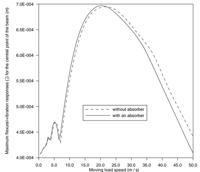
Figure 10 Maximum flexural-vibration responses ( $\bar{y}$ ) for the central point of the beam with and without a two-dof vibration absorber ( $m_a = 16.422 \text{ kg}$ ,  $J_a = 0.2908 \text{ kg.m}^2$ ,  $d = 0.175 \text{ m}$ ,  $k_a = 604120.005 \text{ N/m}$  and  $c_a = 798.692 \text{ Ns/m}$ ).
