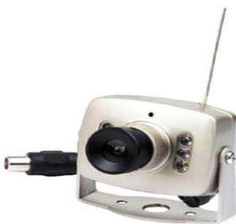
The wireless camera has a night vision which enables no light or low light usage. It performs high-quality picture transmitting and receiving. It can transmit distance up to 200ft. It supports both NTSC and PAL systems. It has output power of 50mW. Its power consumption is less than 400mW with bandwidth of 1.2 GHz and current rating of 500mA and voltage rating of +9V. [8]
