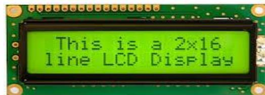
crystals and the liquid crystals do not emit light directly. LCDs are available to display arbitrary images. It displays preset words, digits, and 7-segment displays. It has a wide range of applications including computer monitors, televisions, instrument panels, aircraft cockpit displays.[2]
