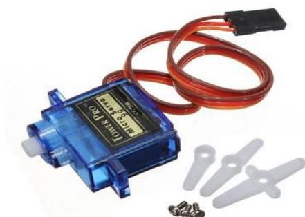
A servo motor is a rotary actuator or linear actuator that allows for precise control of angular or linear position, velocity and acceleration. Servo can rotate approximately 180°. It has an operating voltage of 5V and operating speed of 0.12sec/60° with torque of 1.8 Kg-cm. [7]
