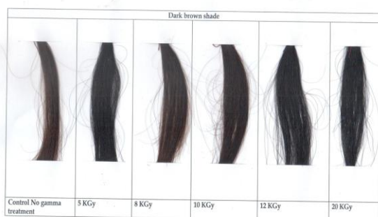
Fig 2: Influence of gamma radiation on colour delivery – Dark brown shade
