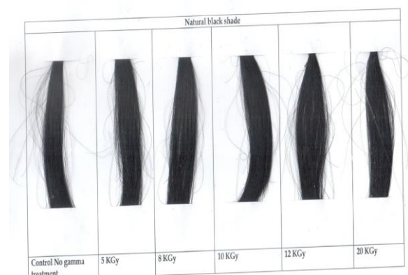
Fig 1: Influence of gamma radiation on colour delivery – Natural black shade
