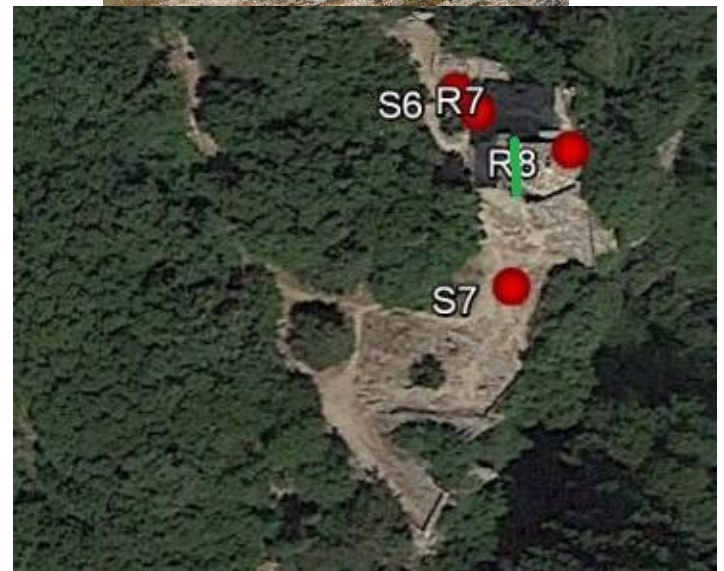
Fig. 8. Montale tower and location of the measurements performed outside the building. The green line indicates the direction of the walls assumed as reference (established NS direction)
