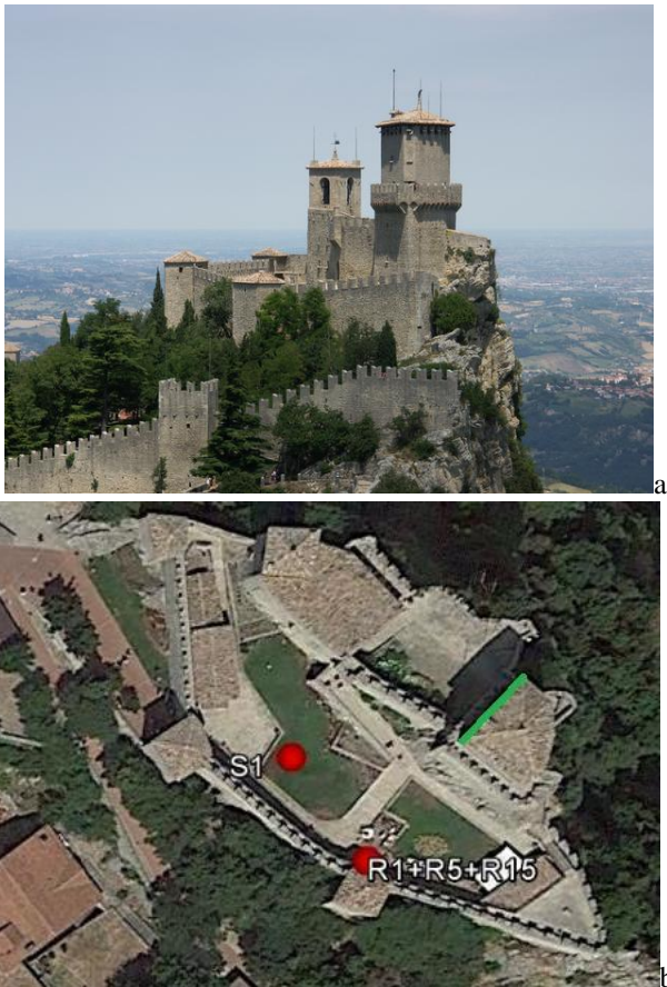
Fig. 2. Guaita tower (a) and location of the measurements performed outside the building (b). The green line indicates the direction of the walls assumed as reference (N-S direction)
