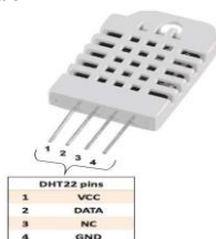
Fig 3: A DHT-22 Sensor
