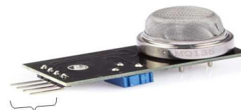
Fig 5: A Typical MQ-135 Sensor
