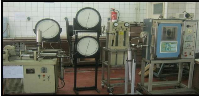
Figure (7): An actual image of slim tube experimental setup (New miscibility lab)
