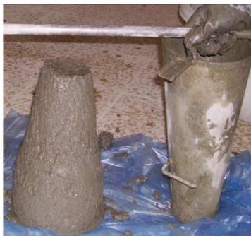
FIGURE III: MAGNETIC WATER FOR SLUMP
