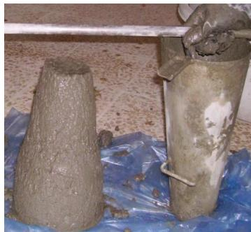
FIGURE III: MAGNETIC WATER FOR SLUMP
