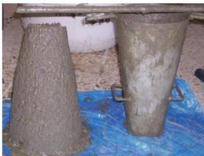
FIGURE II: NORMAL WATER FOR SLUMP
