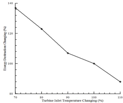
Figure 9. Effect on plant exergy destruction of a change in the turbine inlet temperature
