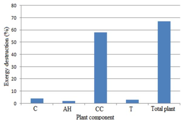
Figure 5. Exergy destruction in components and in total plant in the system
