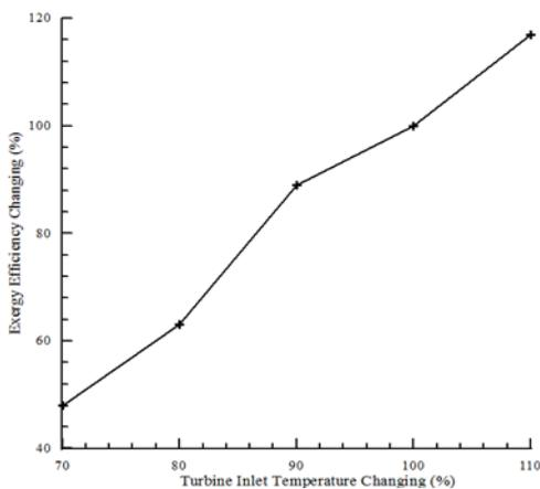
Figure 8. Effect on plant exergetic efficiency of a change in the turbine inlet temperature
