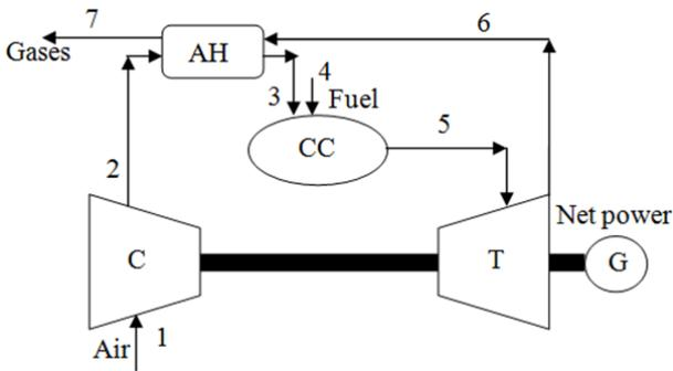
Figure 2. Air pre-heater gas turbine plant
