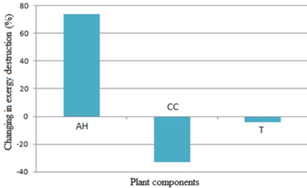
Figure 7. Change in exergy destruction in components due to 120% increase in the turbine inlet temperature
