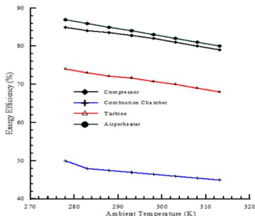
Figure 3. Effect of the ambient temperature on the exergy efficiency of the components of the gas turbine
