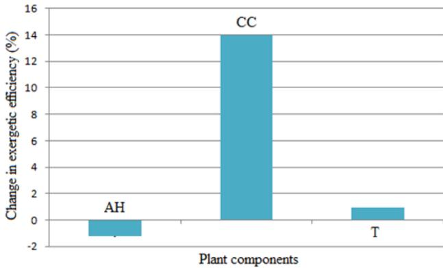
Figure 6. Change in exergetic efficiency of components due to 120% increase in the turbine inlet temperature
