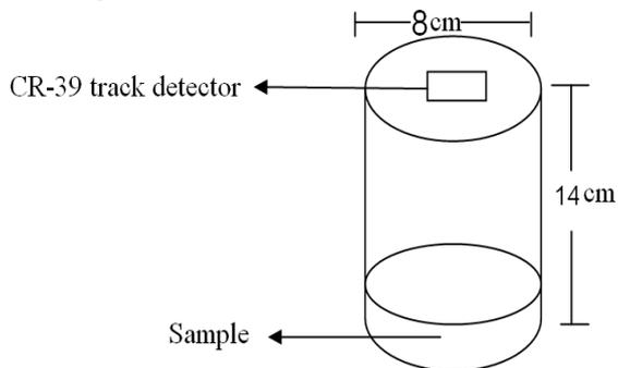
Fig. (2): A schematic diagram of the sealed-cup technique in soil sample.
