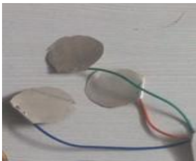
Fig. 2. Silver painted dry electrodes
