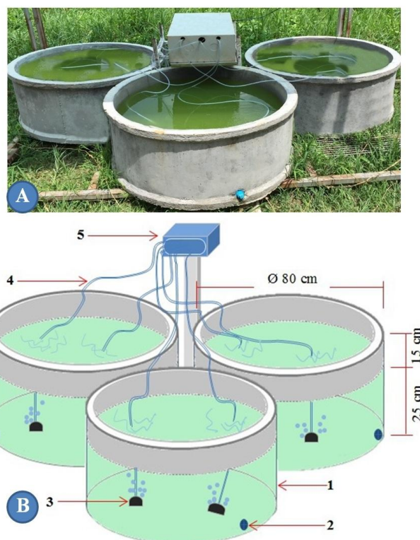
Figure 1 – (A) Open type algal cement pond; (B) - Schematic diagram of algal cement pond: 1. algae growth, 2. outlet of pond, 3. aeration bubble, 4. tube, 5. air pump.
