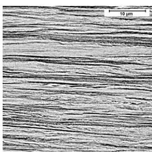
Fig. 2. Material after cold working, specimen no. 1, visible 90% material reduction. SEM
