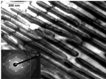
Fig. 7. Specimen no. 5, visible distinct lamellar structure of cementite length scales of the lamellas about 50-80 nm. TEM
