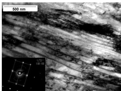
Fig. 3. Magnified area of structure shown in Fig. 2, visible strong plastic deformation of material. TEM
