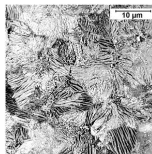
Fig. 4. Material of specimen no. 2, after 15 min long recrystallization annealing visible recrystallized fine-grained structure of pearlitic steel. SEM
