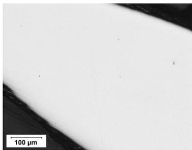
Fig. 1. Specimen No. 1, visible small number of non-metallic inclusions in the form of oxides. Non etched state, LM.
