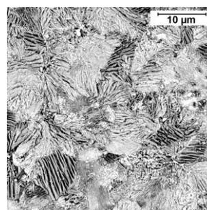
Fig. 5. Structure of material of specimen no. 5 after 60 min long recrystallization annealing, visible distinct lamellar structure of pearlite. SEM
