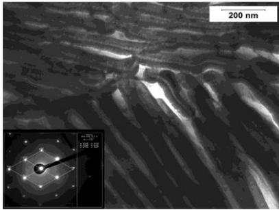
Fig. 6. Specimen no. 2, visible distinct lamellar structure of cementite length scales of the lamellas about 50-80 nm.
