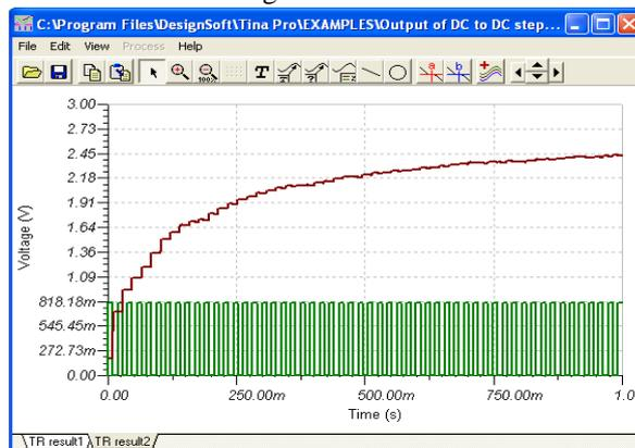
Fig.8 Simulation results of DC-DC step up converter
