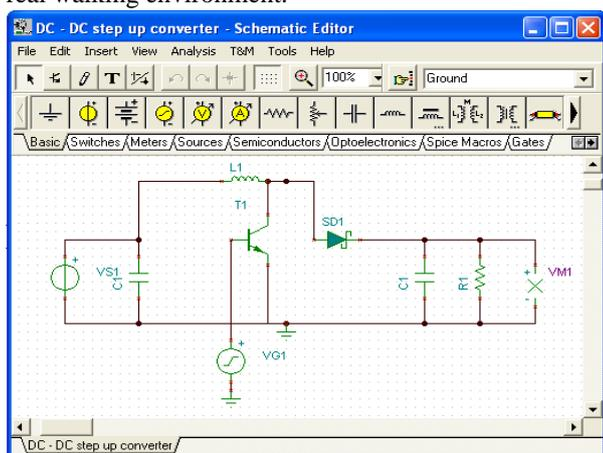
Fig. 7 DC- DC step up converter circuit
