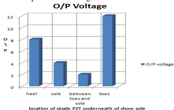
Fig.5 Measurement of o/p voltage at different locations
