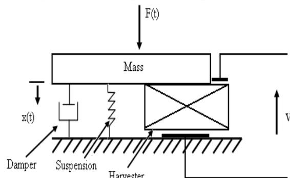
Fig.1 Equivalent model of a vibrating piezoelectric structure
