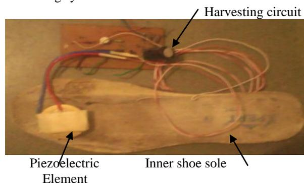
Fig.4 Piezoelectric element locations on shoe sole
