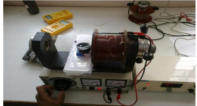
Fig. 1: Experimental set up for Magneto-Rheological Fluid characterization
