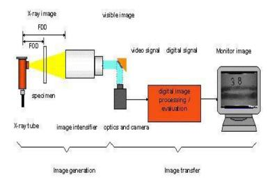
RTR inspection is especially applied for the casting materials, which are produced for automotive, and airplane industry, acceptable defect type and defect size is so a few. Real time radioscopic method has been developed for the last few years and it is widely used in Al wheel production lines.
