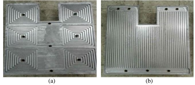
Figure 23. (a) Helical channel and (b) Straight channel cooling plates.
