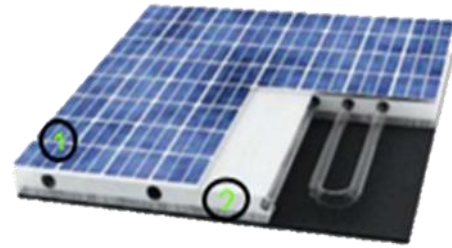
Figure 19. PV panel with Phase-change materials. (1. PV panel, 2. PCM module)
