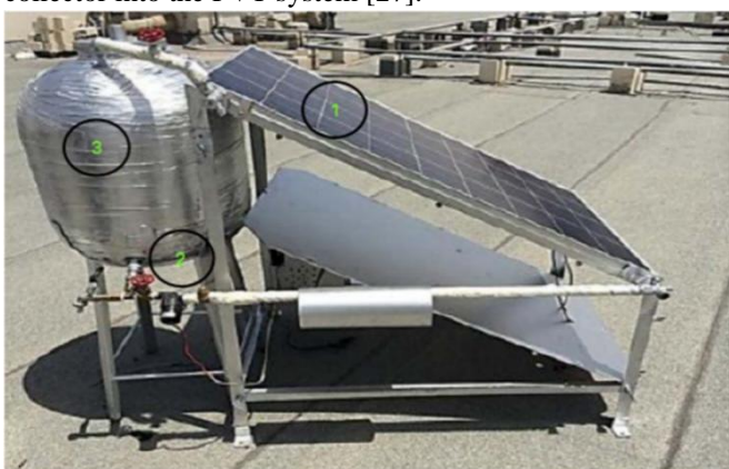
Figure 16. Photovoltaic/Thermal (PVT) system cooled by forced water circulation (1. PV Panel, 2. Circulation pump, 3. Water storage tank with insulation)
