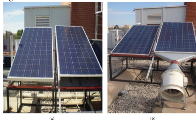
Figure 14. Photovoltaic/Thermal-air system with (a) natural convection and (b) forced air convection configurations [24]
