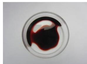
Figure 1. Photograph of a typical used dyeing liquor consisting of an IL and the dissolved disperse dyestuff.
