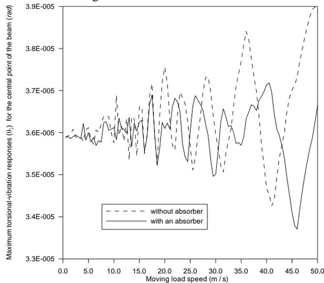
Figure 9 Maximum torsional-vibration responses ( $\theta_x$ ) for the central point of the beam with and without a two-dof vibration absorber ( $m_a = 16.422 \text{ kg}$ ,  $J_a = 0.2908 \text{ kg.m}^2$ ,  $d = 0.175 \text{ m}$ ,  $k_a = 604120.005 \text{ N/m}$  and  $c_a = 798.692 \text{ Ns/m}$ ).
