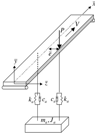
Figure 5 A pinned-pinned beam carrying a two-dof vibration absorber subjected to an eccentric moving force, with magnitude  $P$  and eccentricity  $\bar{e}$ , moving from the left end to the right end of the beam with a constant speed  $V$ .
