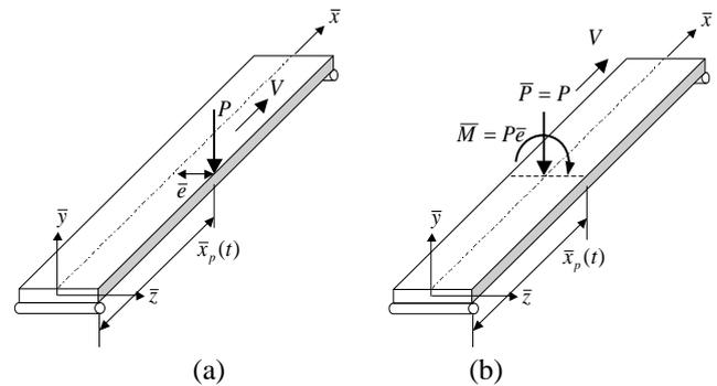
Figure 3 (a) A pinned-pinned beam subjected to an eccentric moving force, with magnitude  $P$  and eccentricity  $\bar{e}$ , can be replaced by (b) the same beam subjected to an equivalent force  $\bar{P} = P$  together with an equivalent moment  $\bar{M} = P\bar{e}$  moving along the centerline of the beam.
