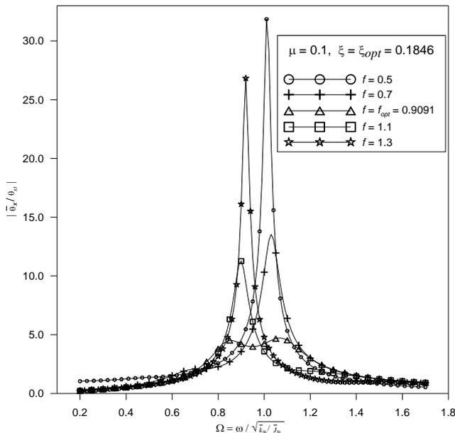
Figure 6 Influence of frequency ratio ( $f$ ) of the two-dof vibration absorber on the dynamic magnification factor  $|\bar{\theta}_x/\theta_{st}|$  of the generalized main vibration system (see Figure 2(a)).
