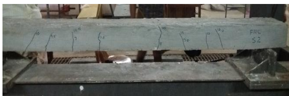
Figure: 6 Crack pattern
