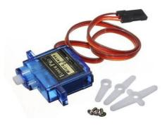
A servo motor is a rotary actuator or linear actuator that allows for precise control of angular or linear position, velocity and acceleration. Servo can rotate approximately  $180^{\circ}$ . It has an operating voltage of 5V and operating speed of 0.12sec/60° with torque of 1.8 Kg-cm. [7]
