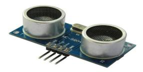
HC-SR04 is the ultrasonic ranging sensor. This economical sensor provides 2cm to 400cm of non-contact measurement functionality with a ranging accuracy that can reach up to 3mm. Each HC-SR04 module includes an ultrasonic transmitter, a receiver and a control circuit. There are only four pins on the HC-SR04: VCC (Power), Trig (Trigger), Echo (Receive), and GND (Ground). [6]
