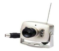
The wireless camera has a night vision which enables no light or low light usage. It performs high-quality picture transmitting and receiving. It can transmit distance up to 200ft. It supports both NTSC and PAL systems. It has output power of 50mW. Its power consumption is less than 400mW with bandwidth of 1.2 GHz and current rating of 500mA and voltage rating of +9V. [8]
