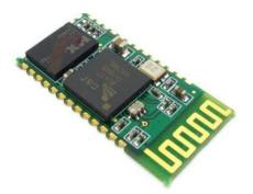
Bluetooth module has a typical -80dBm sensitivity and up to +4dBm RF transmit power. It has a PIO control, UART interface with programmable baud rate, integrated antenna and an edge connector. Its auto-pairing pin is"0000" as default pin and it auto-reconnect in 30 min when disconnected as a result of beyond the range of connection. [3]
