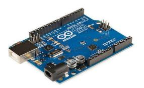
Arduino uno a microcontroller board based on the ATmega328P. It has 14 digital input/output pins (of which 6 can be used as PWM outputs). It also has 6 analog inputs, a 16 MHz quartz crystal, a USB connection, a power jack, an ICSP header and a reset button. It is the most widely used and user friendly microcontroller. Simply connect it to a computer with a USB cable or power it with an AC-to-DC adapter or battery to get started. [1]
