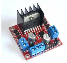
Motor driver is a double H bridge drive chip - L298N with voltage range of 5V-35V and current range of 0-36mA. Maximum power consumption is 25W, dimensions: 43 x 43 x 26mm, weight: 26g and a built-in 5v power supply, when the driving voltage is 7v-35v. [5]
