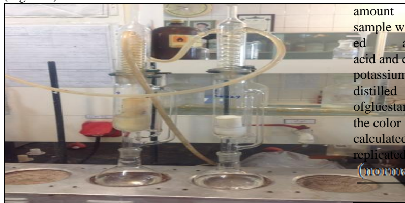
Figure 2 Silybum marianum seed oil extraction by Soxhlet and hexane
