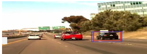
Figure 2: (a,b,c) Tracking results of vehicle for Kalman algorithms. The frames 20, 40 and 80 are displayed.
