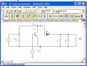
Fig. 7 DC- DC step up converter circuit
